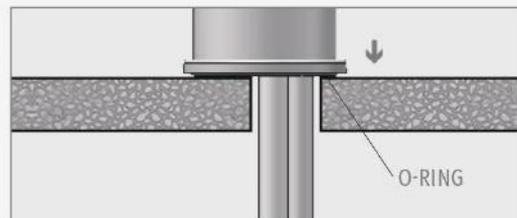
2 Slide the gasket, disk and hexagonal nut over the flexible hose and secure the faucet into place.
